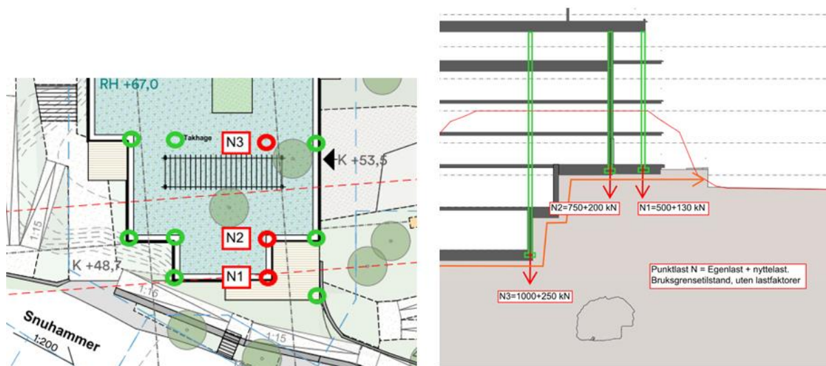
Figure 5-11: Overview of loads in profile BB [4].
